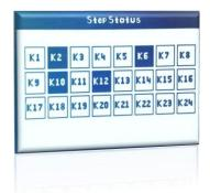
The status of each step (switched ON or OFF) is displayed in this page. The switched ON steps in the example screen are K2, K6, K10 and K12. Others are switched off.
