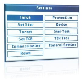
When "Settings" is selected from main page and enter is pressed, a password page will be displayed first. The factory Settings for the password is 0000. Press enter to open the Settings menu.
