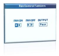
The fan control feature can be activated for cooling of the panel. The FAN ON and FAN OFF values are adjusted by the user.
