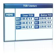
The firing angles and the currents of each branch of star and delta TCR are displayed in this page. The TCR currents are not measured but calculated according to power and angle of the TCR.
