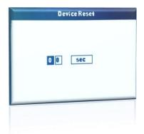
Device reset time is the time that has to elapse to re-start compensation and to set "LOW" to related output when a fault occurs or when a restore occurs following a supply loss.
