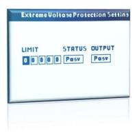
A new screen opens for settings. The "Limit" determines the upper value (lower value for undervoltage) of the protection.
