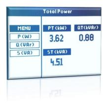
Total active power (PT), total reactive power (QT) and total apparent power (ST) are displayed when first entered this page.
