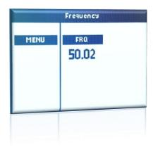
Frequency is displayed referred to phase A, unit is Hz.
