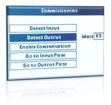
When "Detect Output" is selected and "enter" is pressed, the relay will switch ON and OFF each step one by one.
