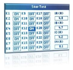
The 24 outputs of the relay can be tested manually. Enter the Step Test page and select the desired step to turn ON or OFF by direction buttons. When pressed enter if the previous position of a step is OFF it will be ON vice versa.
