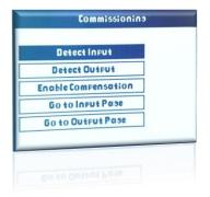
"Detect Input" helps to correct the current order and direction referenced to voltage inputs.
