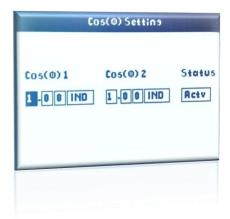
Use the direction buttons to do the settings. If Target Power Factor will be selected as operating mode, the values can be set between 0.01 and 1.00. The power factor can be selected either inductive or capacitive. The status should be selected active. When enter is pressed, the display will return to previous page with updated values and Target Power Factor is the selected operation mode.
