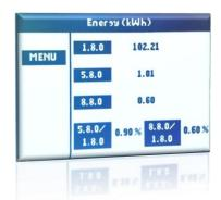
Cumulative import active energy (1.8.0), cumulative reactive inductive energy (5.8.0), cumulative reactive capacitive energy (8.8.0), inductive energy, active energy ratio (5.8.0/1.8.0) and capacitive energy, active energy ratio (8.8.0/1.8.0) are displayed in this page.
