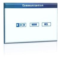
MODBUS RTU protocol is supported by the device. In order to update Modbus parameters, select communication and press enter. Use direction buttons to select the new parameters and press enter.
