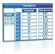
The "counter" column displays how many times a step is switched while the "duration" column display the total switching duration of a step.
