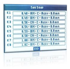
When the Set Step page is selected and enter is pressed, the summaries of settings of the first 8 steps are displayed. To switch the other steps, ">>>" symbol should be selected by direction buttons and enter should be pressed. The next page displays step 9 to step 17 and the last page displays, step 18 to step 24.
