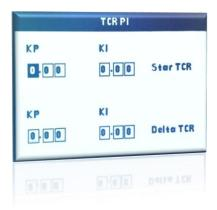
Delta and Star TCR KP and KI parameters can be adjusted from this section.
