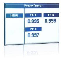
$Cos(\phi)$  value for each phase is displayed in this page. Negative sign means system is capacitive, while positive means the system is inductive.
