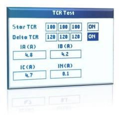
The Delta or Star TCR can be fired manually from this page. The firing angles must be between 90 and 180.
