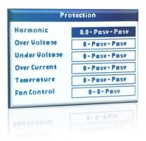
The device has harmonic, overvoltage, undervoltage, overcurrent, high temperature protections and fan control feature.
