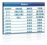
"Events" Page displays the alarms and faults occurred. The conditions of alarms and faults for overvoltage, undervoltage, overcurrent, high THDV and high temperature are set in protection settings page.
