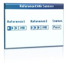
If Target kVAr will be selected as operating mode, the values can be set between 000 to 999 kVAr. The Target kVAr value can be selected either inductive or
