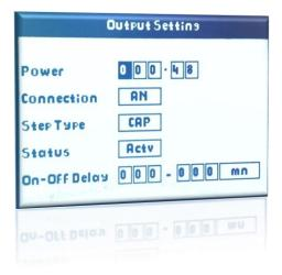
Each steps setting is done individually. If any of the settings wanted to be changed, that step should be selected. A "step setting" screen is displayed when enter is pressed.
