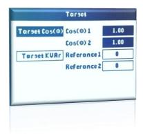
Two target operation modes are selectable: Target Power Factor or Target kVAr.
